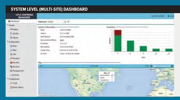
The system level dashboard presents a map view of all the sites with inventory details for immediate visualization of the entire network. The site-level dashboard allows you to see the status of your access points and their radios, the client devices — including device type — connected to your access points, how much capacity is available and more. And a drop-down box allows you to view information for your preferred timeframe — for the last 30 minutes, the past two hours or the last 24 hours.
