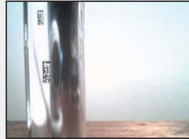
Rectangular Laser Marks on Shiny Curved Surface
