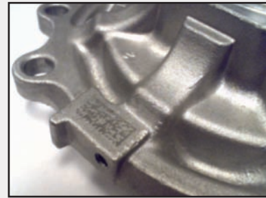
Rectangular Laser Marks on Shiny Curved Surface
