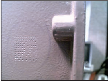
Painted Over Peen Mark Shows How Dots light up from Angle Lighting
